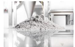
**VESTAKEEP® 2000 FP** is an unreinforced, medium-viscosity polyether ether ketone fine powder. It can be used as a basic resin or in blends with different additives for manufacturing compression molding parts.
